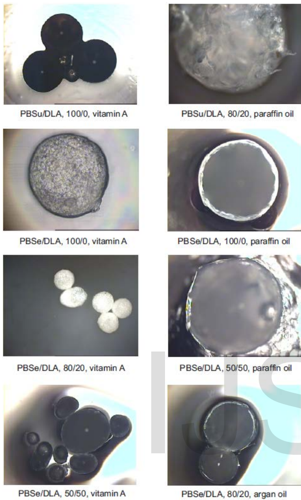
Fig. 4. Images from polarization microscope microcapsules with different filling.
